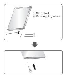
9. Change screw hole covers on middle cover plate from left to right (as shown in figure below).
