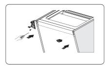
12. Transfer the lower door to the property position, adjust the lower hinge part, make the hinge axis into the lower hole of the lower door, then tight the bolts.
