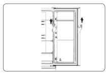
6. Place the upper door on a smooth surface with its panel upwards. Loose screw ② and part ①, then Install them to the left side and tighten securely.
